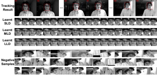
Figure 3. Online dictionary learning for template update. Line 1: tracking results; Line 2-4: examples of the learned dictionaries at frame 100; Line 5-7: collected negative samples used for the discriminative observation model (see Section 3.3).
